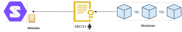
Figure 5: Storing the metadata of an ERC721 token smart contract in Solid pod
